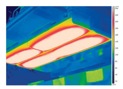
The heat is distributed above the screed plate, ensuring even temperatures front to back and side to side.
